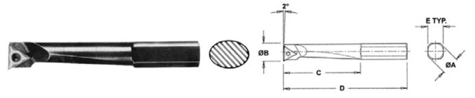
For added strength and rigidity, the quill portion of the shank is oval shaped. In addition to providing greater chip clearance, this design helps eliminate tool deflection, resulting in better cutting performance.
