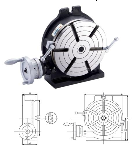
The work table is graduated 360 degrees around it's circumference and is driven by a precision worm and gear providing a 90:1 reduction ratio. One turn of the handle moves the table through four degrees. The dial is graduated in divisions of 1 minute and the vernier scale allows readings down to 10 seconds.
