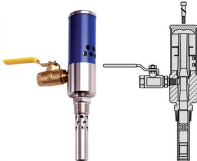
The Royal Pnevac pump is a simple, low-cost device that generates a strong vacuum when compressed air flows through its internal venturi.
